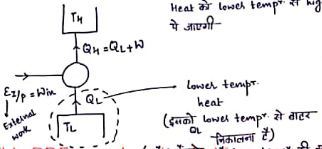
$$\rightarrow (\text{COP})_{\text{Ref.}} = \frac{Q_L}{W} \quad \text{for finding the performance of Refrigeration system}$$
